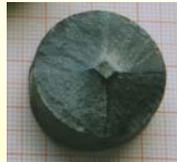
World record 2001: 16 Tesla in superconducting permanent magnets
